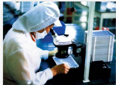
Crystal Blank Inspection
